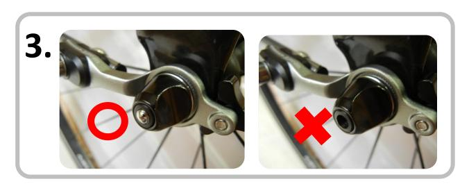
Check 3: Rear/front wheel QR axle is requested to appear on the QR nut hole in order to make the fender bracket safely installed well. If not to see the QR axle appearing on the QR nut hole, it means no enough space for fender installation on frame dropouts. To avoid to pose a crash hazard, the rear/front QR axle in enough length is a must for safety installation of the fender bracket.
