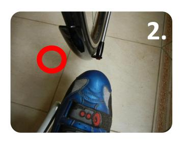
Check 1: Dropout diameter larger than 29.0mm is not fitting to fender installation.
